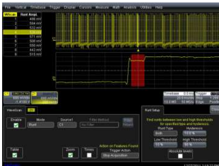
Figure 4: A Runt trigger is used to find a signal integrity problem in a CAN signal. A long set of data is captured in the top trace. Nine faults are found. The fourth one is zoomed for detailed viewing in the lower trace
