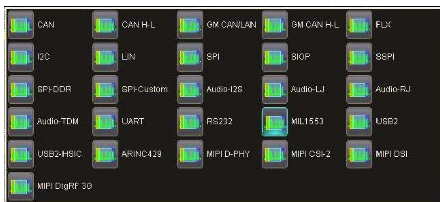
Figure 1: LeCroy oscilloscopes can capture and decode a wide variety of low speed serial data protocols
