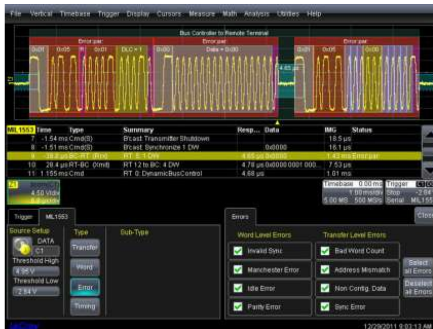
Figure 8: Protocol Aware Triggering and Bus Decode. In this case the scope is triggering on Error conditions
