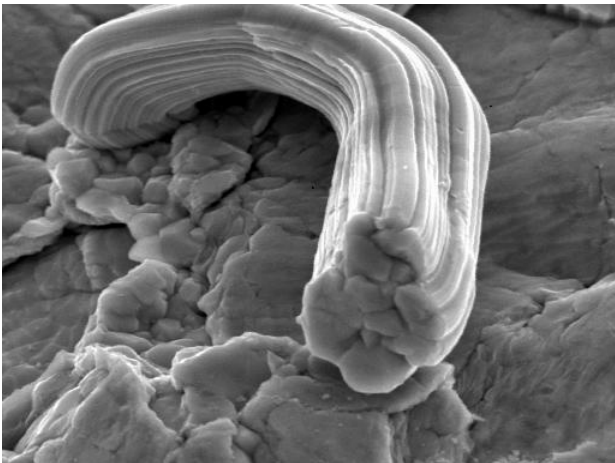
Tin whisker filament with striations.
