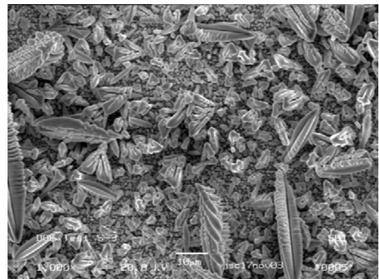
Dendrites formed on a tin surface during plating. These are not tin whiskers.
