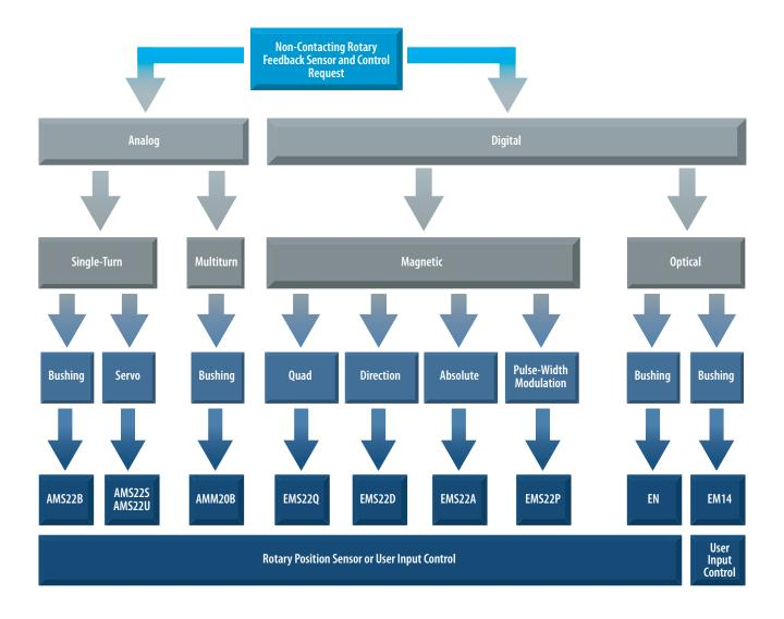
In selecting a rotational control or position feedback sensor for a given application, the most important characteristics to consider are the technology type, output signal, and expected cycle life of the product. The flow chart above is provided to assist in selecting the product best suited for a given application.
