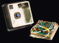
Small form-factor opto-electronic media converter with field fault monitoring
