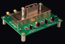
HiPer-D connector with size #8 opto-electronic contacts evaluation board
