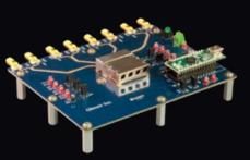
**PCB-mount transceiver** evaluation board
