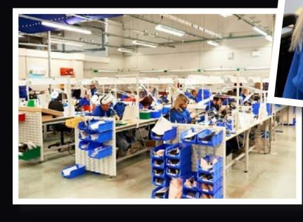
The Glenair Mansfield clear room assembly area is used for fabrication of laser, space, and satellite assemblies **IAW ISO Class 8** -100,000 PPM
