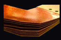
26 layer EMI/RFI shielded rigid flex assembly
