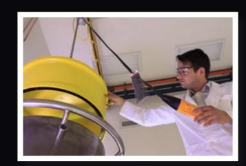
SeaKing<sup>™</sup> and SuperG55<sup>™</sup> QUALIFICATION TESTING: Both Glenair Series 70 SeaKing and SuperG55 rugged dry-mate subsea connectors have been tested and qualified to their 10K psi pressure rating—open-face and mated—in Glenair's state-of-the-art hydrostatic test lab. Additional testing included mating cycles, salt spray, and electrical continuity.
