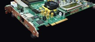
Ruggedized FMC connectivity PCBA for Ethernet, Fiber channel, and/or DVI, SMPTE video system applications
