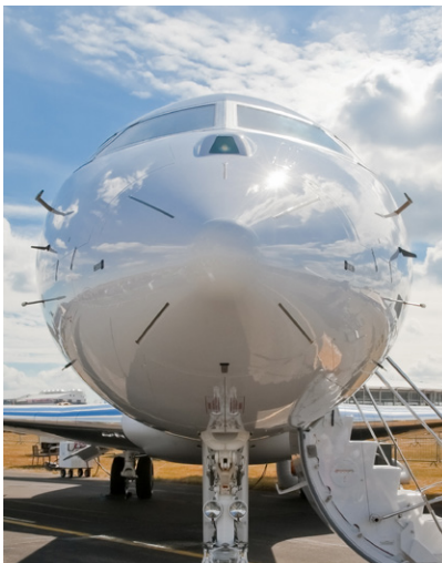
Lightning diverter strips on the nose of an airplane
