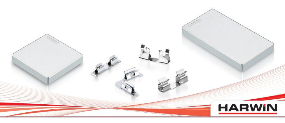
Harwin's SMT Clip and Can system works by soldering the Clips to the PCB during the SMT phase. The Cans are then pushed into the clips in a very quick secondary operation.
