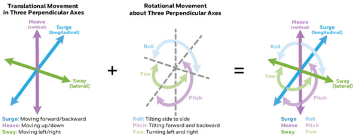
The Honeywell TARS Series ruggedized IMUs measure six degrees of freedom. (Image courtesy of Honeywell.)
