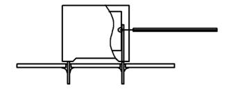
Temperature monitored inside the capacitor.
