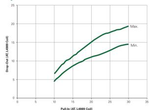
$\textbf{Note:} \ \textbf{Chart represents the range of Drop-Out, min to max for a given Pull-In value.}$
