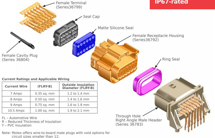
Mating configuration of a typical 2-by-6 circuit, sealed MX120G™ wire-to-board assembly (exploded view)
