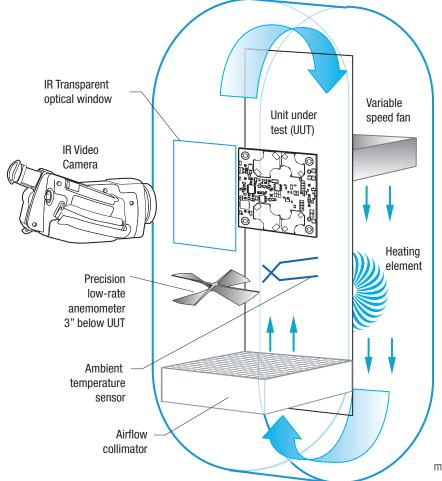
Figure 7. Vertical Wind Tunnel
