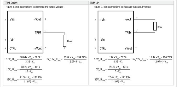
Accuracy of adjustment is subject to tolerances of resistors and factory adjusted output accuracy. Vout is equal to the desired output voltage.
