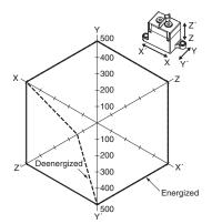
The value at which malfunction occurred was measured after applying shock to the test piece 3 times each in 6 directions along
