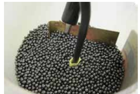
Figure 6 - Dielectric Strength Test - PLASTI-GRIP Terminal
