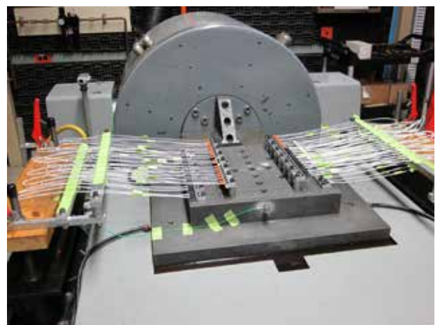
Figure 3 - Military Vibration Test - PIDG Terminals
