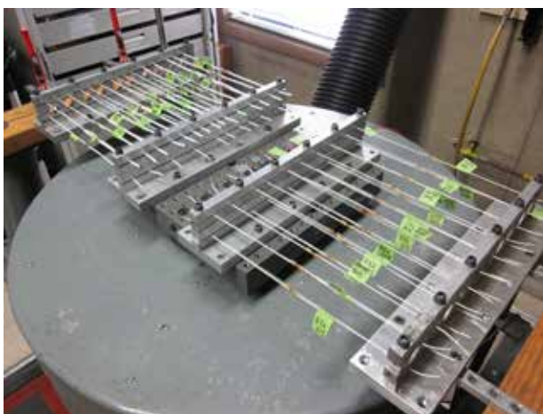
Figure 2 - Military Vibration Test - SOLISTRAND Splices
