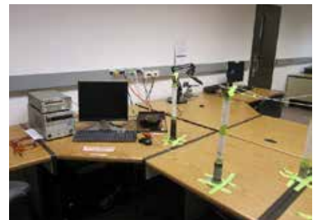
Figure 7 - Millivolt Drop Test - SOLISTRAND
