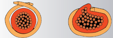
Insulation is not securely held
